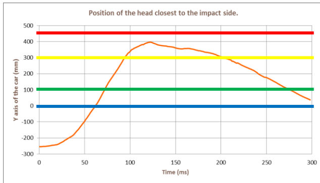
Fig.13 Plot showing the displacement in the Y axis of the dummy head respect to the coordinate system of the vehicle in a far side test. Presented data has been modified for public purpose.
