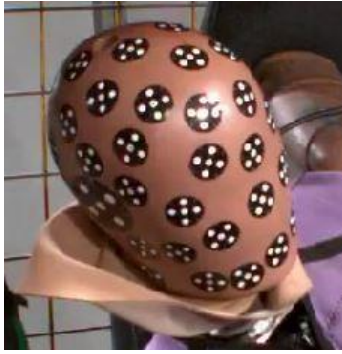
Fig.10 MXT marker position on the dummy head.
