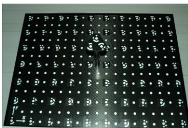
Fig.5 Rigid carbon fiber board used in IDIADA for photogrammetric calibration.
